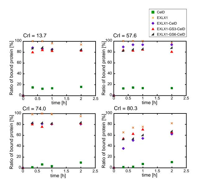
**Fig. 4** Time courses of the ratio of bound protein to cellulose with different CrI. Cellulose concentration (5 g/L) and protein concentration (1.0  $\mu$ mol/L) were same in all experiments.
