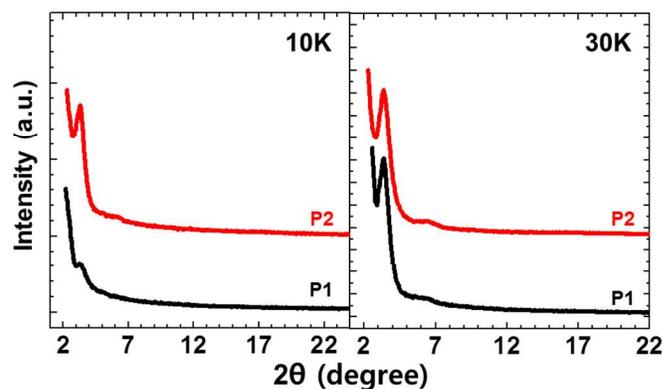
**Figure 2.** GIXRD measurements obtained from the P1 and P2 polymer films, for molecular weights of 10 kg/mol (a), or 30 kg/mol (b).
