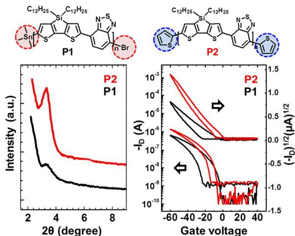
The ends of conjugated polymer chains were capped with thiophene units to enhance intermolecular packing and decrease device hysteresis by removing charge trap sites.
