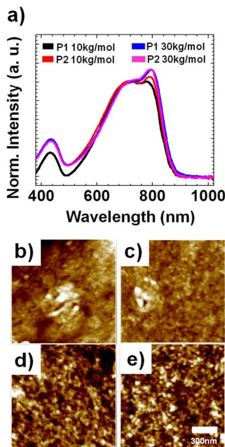
**Figure 1.** UV-vis. spectra of P1 and P2 films prepared from polymers with different molecular weights (a), and AFM height images of films corresponding to 10 kg/mol P1 (b), 10 kg/mol P2 (c), 30 kg/mol P1, (d) and 30 kg/mol P2 (e). The scale bars in the AFM images indicate 300 nm.
