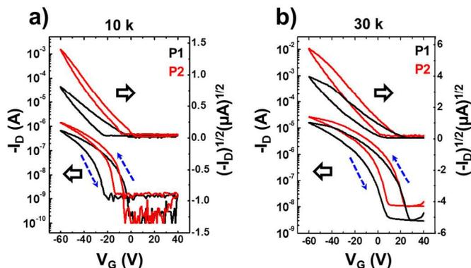
**Figure 4.** Plot of  $I_D$  versus  $V_G$  at a fixed  $V_D$  of  $-60 \text{ V}$ , on both the linear (right axis) and log (left axis) scales, for P1 and P2 OFETs prepared with polymers having two different molecular weights: 10 kg/mole (a) or 30 kg/mole (b).
