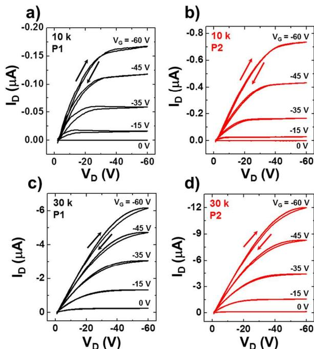
**Figure 3.** The output characteristics of OFETs prepared using the P1 or P2 polymers with either low or high molecular weights, with operation at various gate voltage ( $V_G$ ) between 0 V and -60 V. The arrows represent the scan directions.
