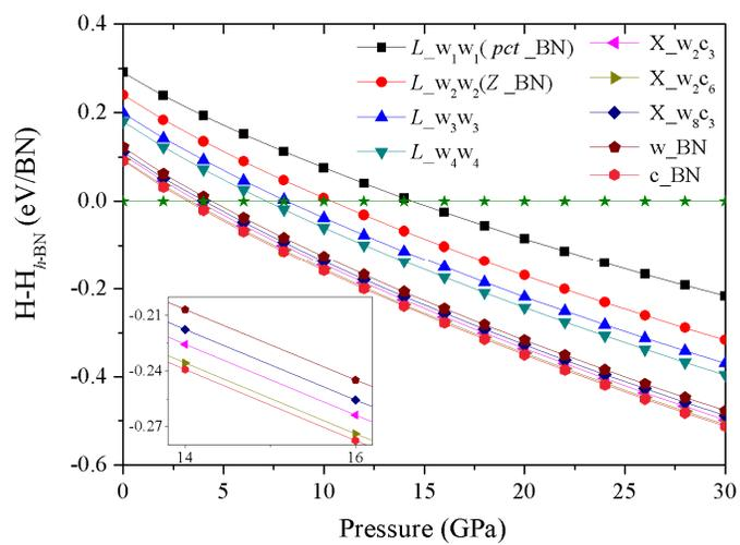
Figure 3. Calculated enthalpy difference per BN pair with respect to *h*-BN for numerous BN allotropes versus pressure.
