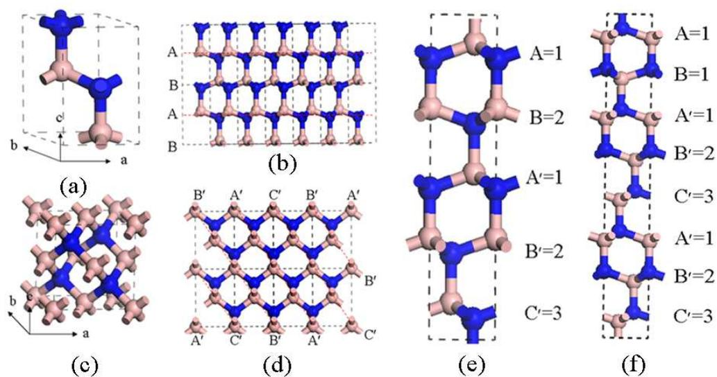
Figure 1. (a) and (c) illustrate the crystallographic structure of the w-BN and c-BN. (b) and (d) show the 2D projections of the  $6 \times 1 \times 2$  supercell of w-BN along  $(1, 1, 0)$  direction and of the  $3 \times 2 \times 1$  supercell of c-BN along  $(1, 0, 1)$  direction. (e) and (f) show the 2D projections of the unit cell of  $X-c_3w_2$  and  $X-c_6w_2$  respectively.
