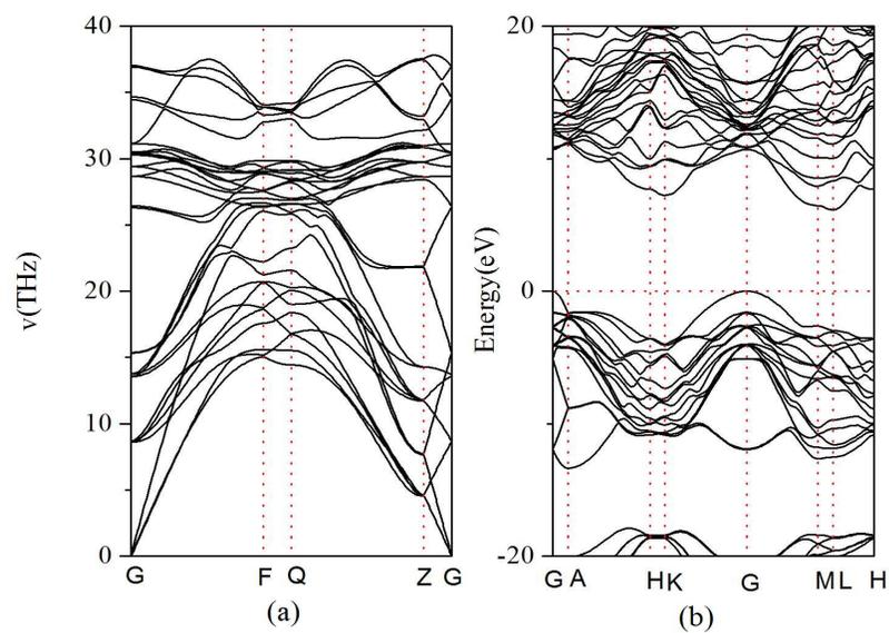
Figure 4. Properties of the X-w<sub>2</sub>c<sub>3</sub> phase. (a) Calculated phonon dispersion curves of X-w<sub>2</sub>c<sub>3</sub> phase at 0 GPa. (d) Calculated electronic band structure at zero pressure.
