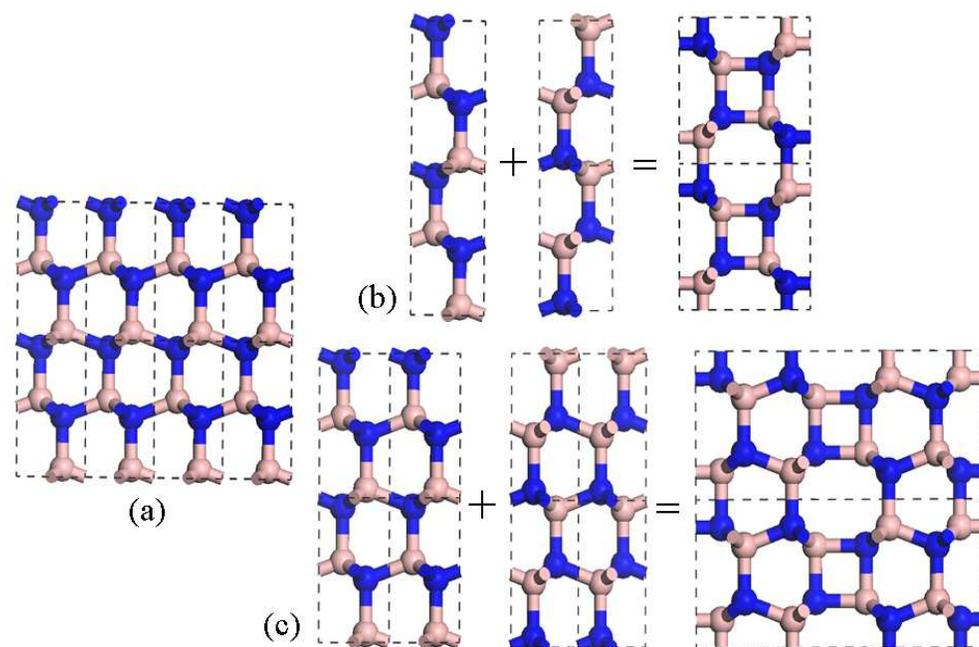
Figure 2. (a) shows the 2D projections of the  $4 \times 1 \times 2$  supercell of w-BN along  $(1, 1, 0)$  direction. (b) and (c) show the combination of the  $X-w_1w_1$  BN phase and  $X-w_2w_2$  BN phase, respectively.
