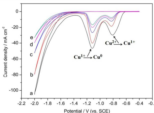
**Fig. 4** Cyclic voltammograms recorded at sample a-e in CO<sub>2</sub>-saturated 0.2M KI aqueous solution at a sweep rate of 0.1 V/s at 25°C.
