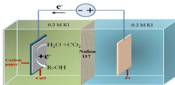
Morphology-controlled CuO nanoparticles for electroreduction of CO<sub>2</sub> with an excellent selectivity for ethanol.
