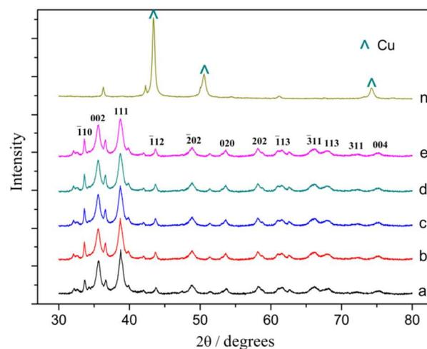
**Fig.1** a-e: X-ray diffraction (XRD) patterns of CuO nanoparticles before electrolysis of sample a-e, n: sample a after 1 h electrolysis.
