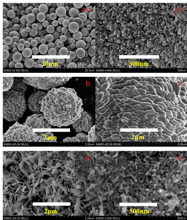
**Fig. 2** FE-SEM patterns of CuO nanoparticles. (a-1), (a-2): sample a; (b)-(e): sample b-e.
