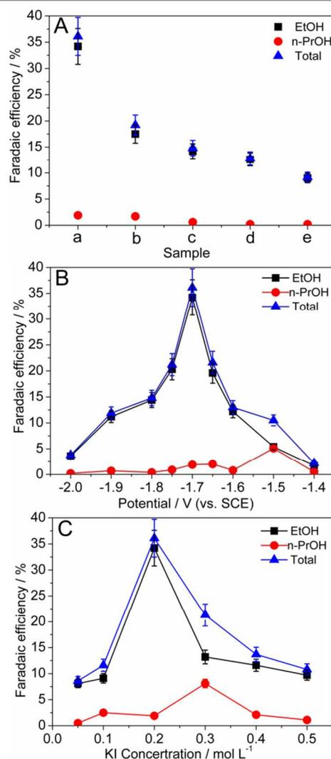
**Fig. 3** Electroreduction of  $\text{CO}_2$  under multiple conditions. A: effect of different electrodes (sample a-e),  $-1.7\text{ V}$ ,  $0.2\text{ M KI}$ ; B: effect of potential,  $0.2\text{ M KI}$ ; C: effect of KI concentration,  $-1.7\text{ V}$ .
