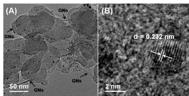
Figure 1. (A) TEM and (B) HRTEM images of PdAu/GNs-CB.
