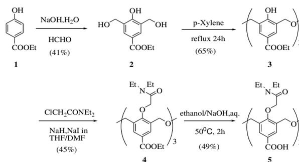
Scheme 1. Synthesis of hexahomotrioxacalix[3]arene *cone*-5.
