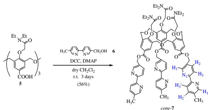
**Scheme 2.** Synthesis of hexahomotrioxacalix[3]arene *cone-7*.
