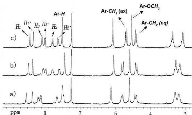
**Fig. 3.** Partial  $^1\text{H}$  NMR titration of *cone-7*/guest complex ( $\text{H}/\text{G} = 1:1$ ); a) free *cone-7*; b) *cone-7*  $\supset$   $\text{AgClO}_4$ ; c)  $\text{LiClO}_4 \subset [\text{cone-7} \supset \text{Ag}^+]$ ; Solvent:  $\text{CDCl}_3/\text{CD}_3\text{CN}$  (10:1, v/v).
