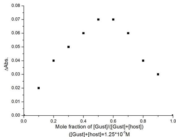
**Fig. 8.** Job plot of the extractions of Ag<sup>+</sup> with host *cone-7*.
