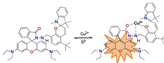
**Scheme 2** Proposed mechanism for the fluorescent changes of sensor **RB-SP2** upon the addition of  $\text{Cu}^{2+}$  and  $\text{S}^{2-}$
