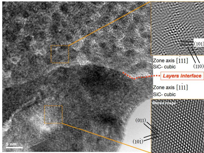
Fig. 3. HRTEM analysis of the silicon carbide nanoparticles introduction into porous polymer coatings.
