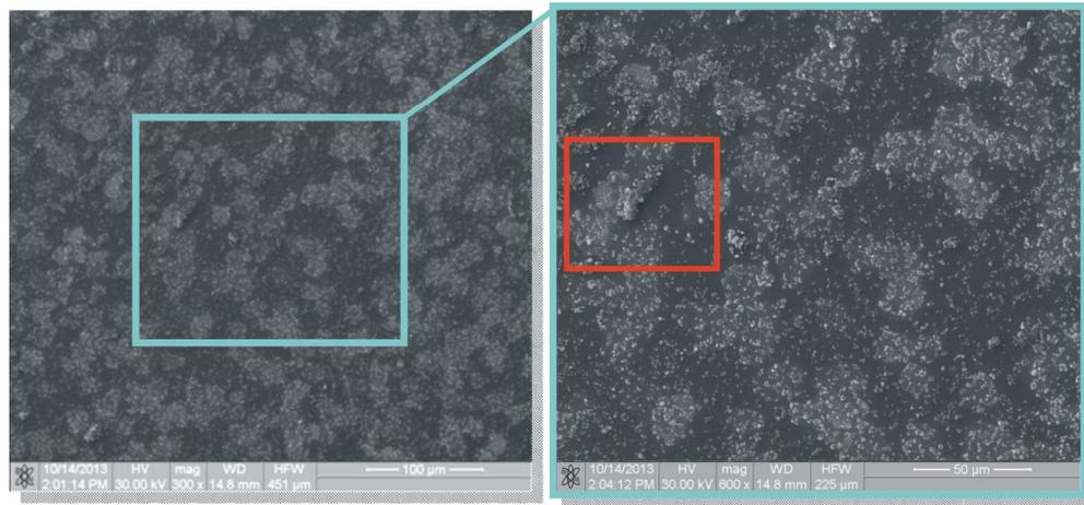
Fig. 1. Example of SEM images of nanoparticles distribution in PEM – smaller frame indicates area used for FIB thin foil preparation.
