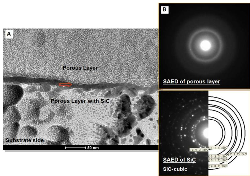
Fig. 2. Cross section TEM analysis of the silicon carbide nanoparticles introduction into porous polymer coatings: a) bright field image; b) selected area electron diffraction patterns. The red arrow indicates a border between polymer porous layers.
