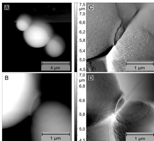
**Figure 6.** AFM images of *Pichia pastoris* (A) overview scan - height image (B-D) single cell scan – (B) height image (C) amplitude image (D) phase image.
