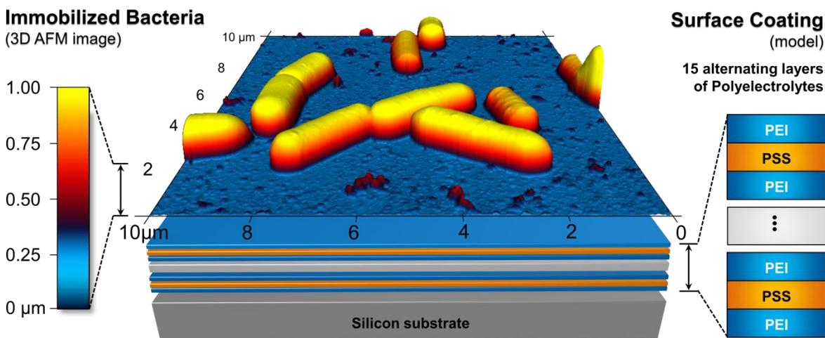
Atomic force microscopy image of immobilized bacteria (*Lysinibacillus sphaericus* JG-B53) on polyelectrolyte supported surface and model of layer constitution of new immobilization matrix.
