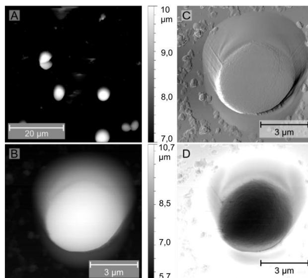
**Figure 7.** AFM images of *Chlorella vulgaris* (A) overview scan - height image (B-D) single cell scan – (B) height image (C) amplitude image (D) phase image.
