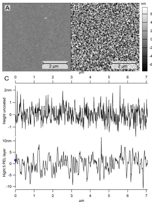
**Figure 3.** AFM images of silicon substrates; (A) AFM scan of plain silicon wafer, (B) AFM scan of silicon wafer after applying 15 polyelectrolyte layers, (C) Surface profile of uncoated and coated silicon wafer derived from the AFM images (A) and (B) measured from the lower left to the upper right corner.
