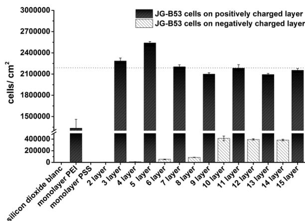
**Figure 2.** Total cell numbers representing effects of polyelectrolyte coatings on silicon dioxide surfaces to the bacterial cell adhesion of *Lysinibacillus sphaericus* JG-B53. Total adsorbed cells were normalized to one square centimeter depending on different constituted PE mono- and multilayer.
