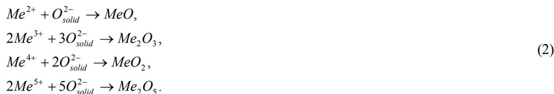
Also, direct ejection of metal into the electrolyte can occur through microdischarge channels during the breakdown:<sup>4</sup>
