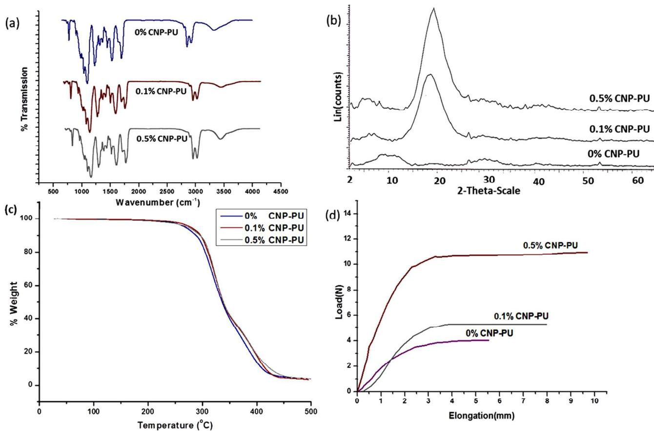
Fig. 5 (a) FTIR spectra (b) XRD graph (c) TGA analysis and (d) UTM analysis of 0%, 0.1% and 0.5% polyurethanes.
