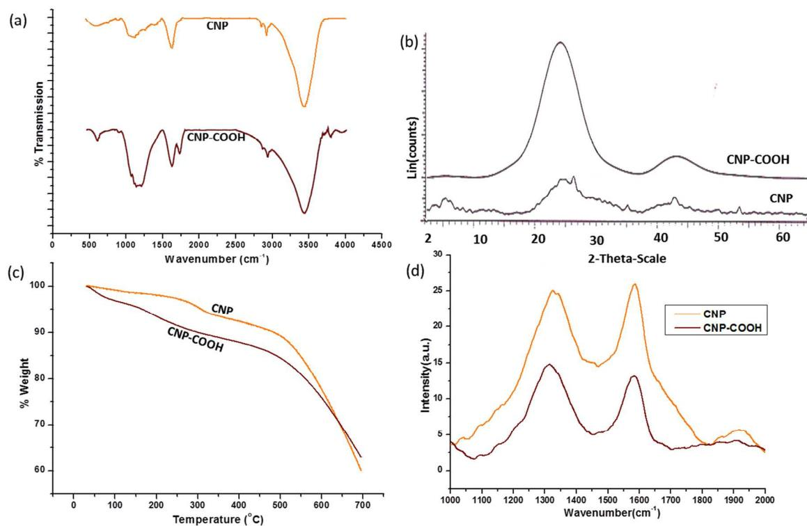
**Fig. 2(a) FTIR (b) XRD graph (c) TGA graph (d) Raman analysis of CNP and CNP-COOH incorporated polyurethane.**
