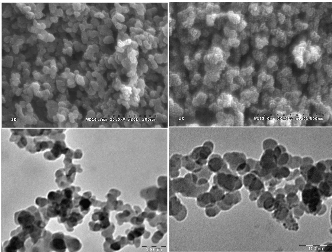
**Fig. 1 FESEM images (above) and TEM images (below) of graphitic-carbon nanoparticles and piranha solution treated carbon nanoparticles (from left to right)**
