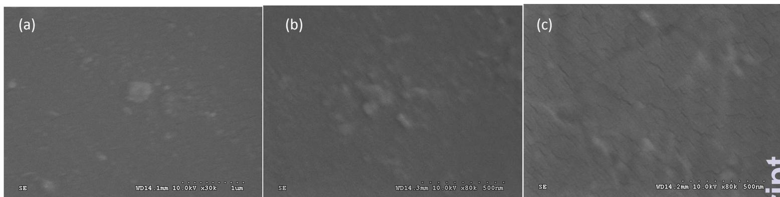
**Fig.6 FESEM images of (a) Neat polyurethane (b) 0.1wt% CNP-COOH incorporated polyurethane and (c) 0.5wt% CNP-COOH incorporated polyurethane.**
