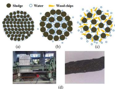
Schematic mechanism of the effect of adding wood chips on sludge dewatering: (a) sludge without conditioning; (b) sludge with chemical conditioning; (c) sludge with chemical and physical conditioning; and (d) a physical image of a dewatered sludge cake with wood chip conditioning
