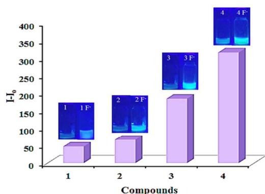
**Fig. 5** Compounds **1**, **2**, **3** and **4** showing  $I_f$ ;  $I_f$  is final fluorescence intensity after addition of 1 mmol of  $F^-$  ions and  $I_0$  is initial fluorescence intensity of compounds. Insets show the changes in respective compounds on addition of  $F^-$  ions under 365 nm illumination.
