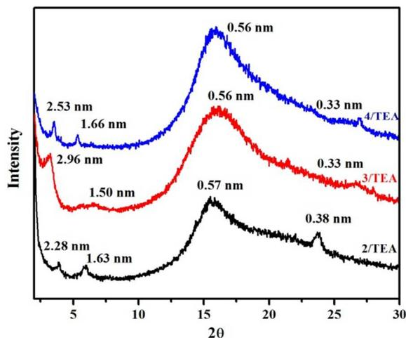
Fig. 4 X-ray diffraction patterns of xerogels **2**, **3** and **4** obtained from triethylamine (TEA).
