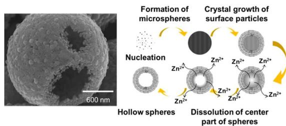
ZnO hollow microspheres exhibiting only *c* planes on the surface were successfully synthesized by a solvothermal method even without using template. The ZnO hollow microspheres are formed by preferential dissolution of centers of ZnO solid microspheres which have low crystallinity.
