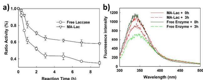
**Figure 4.** Deactivation of free and modified laccases in acidic condition (pH 3.5); a) Deactivation plot; b) Fluorescence emission spectra.
