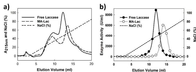
**Figure 1.** Anion-exchange chromatography of free and modified laccase on HiTrap DEAE FF (1ml columns); a) Protein content of the elution; b) Laccase activity of the elution.
