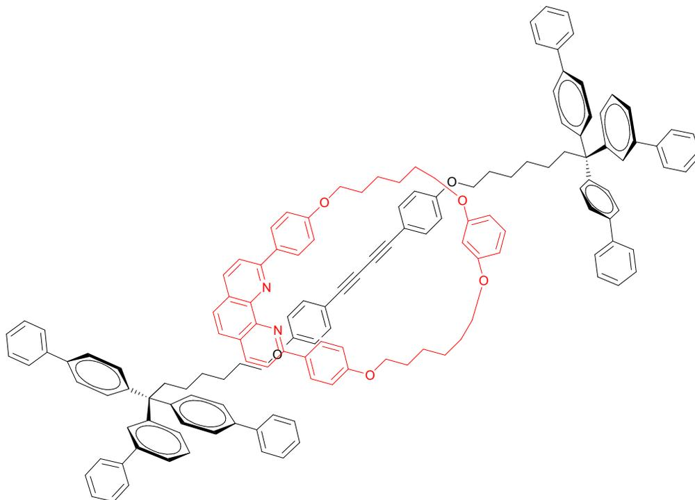
**Fig 6** [2]rotaxanes from a macrocyclic Cu(I)-phenanthroline complex. Reprinted with permission from ref. 99, copyright 2006, American Chemical Society.
