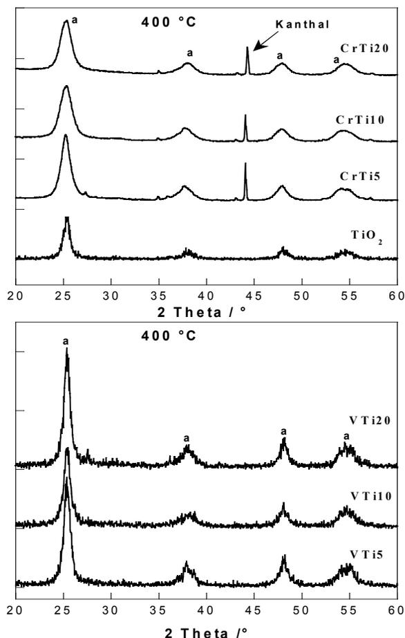
Fig. 4 X-ray diffraction (XRD) patterns of MTiX; a: anatase
