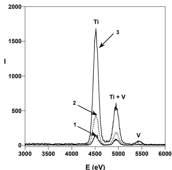
Fig. 6 EDX analysis of different zones of the  $\text{VTi20}$  sample.
