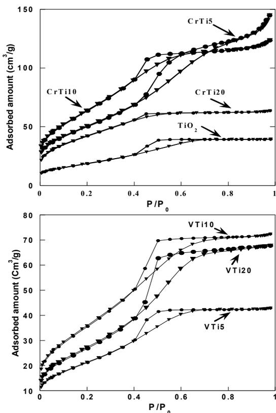
Fig.1 Isotherms for adsorption of nitrogen on MTiX samples
