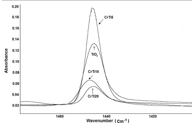
Fig. 2 IR adsorption spectrum of pyridine for CrTiX; evacuation at 150°C.
