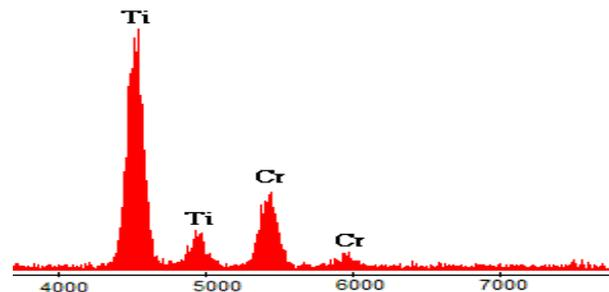
Fig. 5 EDX analysis of zone 3 of the  $\text{CrTi20}$  sample.
