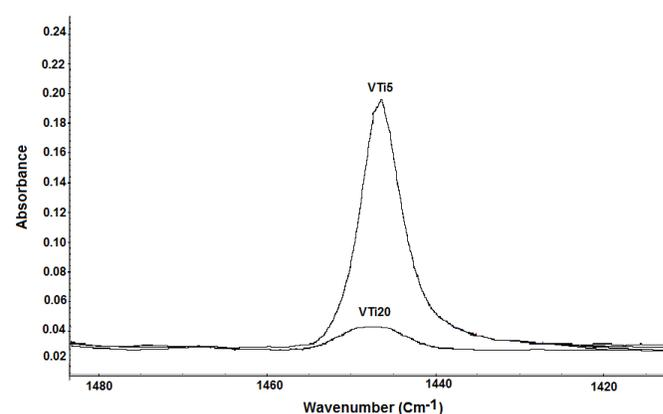
Fig. 3 IR adsorption spectrum of pyridine for VTiX; evacuation at 150 °C.
