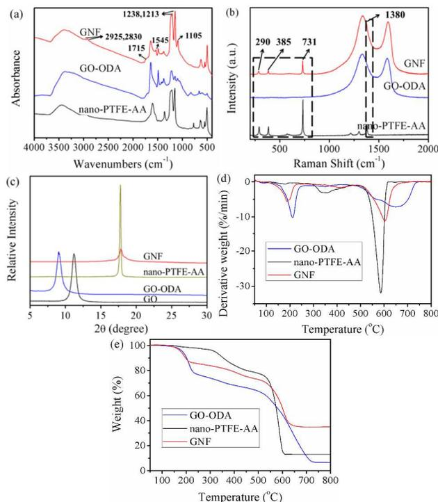
**Fig. 3** (a) FTIR spectra, (b) Raman spectra (excitation wavelength 631 nm), (c) XRD patterns, (d) DTG curves and (e) TGA thermograms of nano-PTFE-AA, GO-ODA and GNF.
