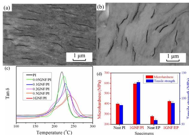
**Fig. 8** TEM images showing GNF dispersion of (a) 1GNF/PI and (b) 1GNF/EP specimens. (c) Damping spectra of PI and GNF/PI composites films. (d) Microhardness and tensile strength of neat PI, 1GNF/PI, neat EP and 1GNF/EP specimens.
