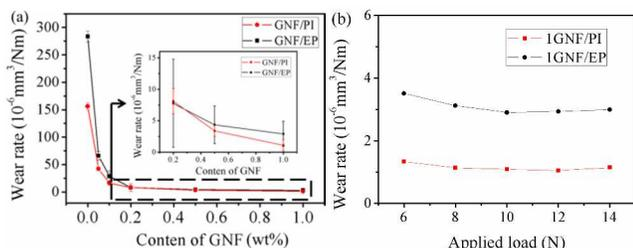
**Fig. 6** (a) Relationship of wear rate of GNF/PI and GNF/EP specimens with different GNF content. The inset shows its corresponding enlarged view. (reciprocating frequency: 10 Hz, sliding distance: 480 m, load: 10 N, RH: 40%). (b) Relationship of wear rate of 1GNF/PI and 1GNF/EP specimens with different applied load (reciprocating frequency: 10 Hz, sliding distance: 480 m, RH: 40%).
