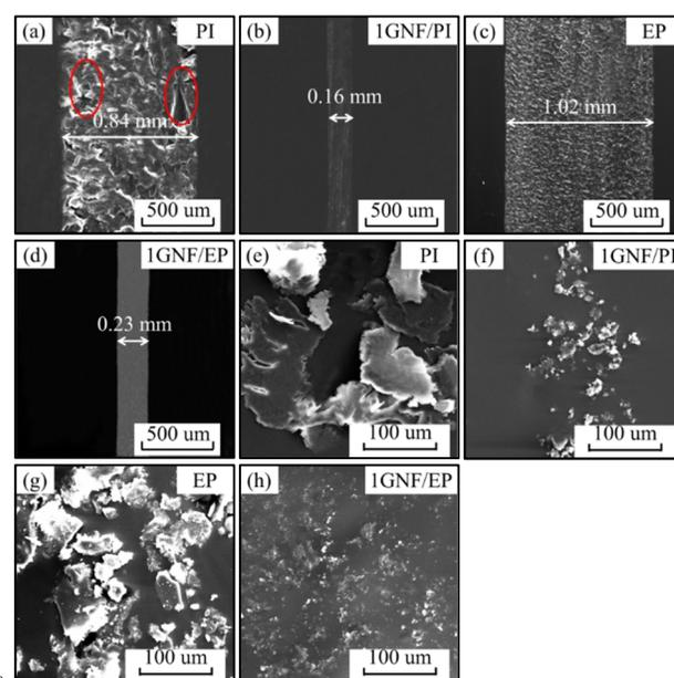
**Fig. 9** SEM images of worn surfaces and wear debris of (a), (e) neat PI, (b), (f) 1GNF/PI, (c), (g) neat EP and (d), (h) 1GNF/EP specimens.
