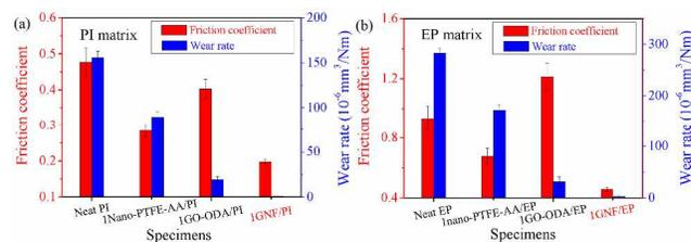
**Fig. 7** Comparisons (a) tribological properties of neat PI, 1nano-PTFE-AA/PI, 1GO-ODA/PI and 1GNF/PI specimens, and (b) tribological properties of neat EP, 1nano-PTFE-AA/EP, 1GO-ODA/EP and 1GNF/EP specimens. (reciprocating frequency: 10 Hz, sliding distance: 480 m, load: 10 N, RH 40%).
