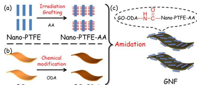
**Fig. 1** Covalent compounding between GO and nano-PTFE including (a) irradiation grafting of nano-PTFE with AA, (b) chemical modification of GO with ODA and (c) preparation of GNF by amidation reaction between GO-ODA and nano-PTFE-AA.
