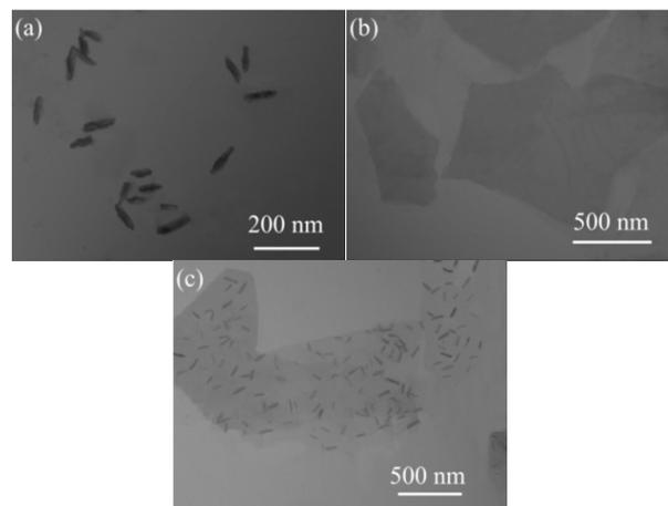
**Fig. 4** TEM images of (a) nano-PTFE-AA, (b) GO-ODA and (c) GNF.
