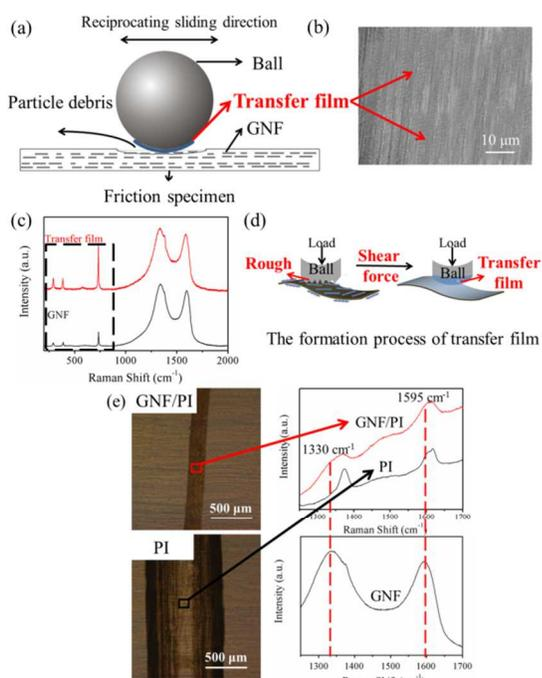
**Fig. 10** (a) A schematic for tribological mechanism of GNF/polymer composites. (b) SEM image of transfer film on the counterpart. (c) Raman spectral comparison between transfer film and GNF. (d) The formation process of transfer film. (e) Raman analysis of worn surface of GNF/PI and PI specimens after washing.
