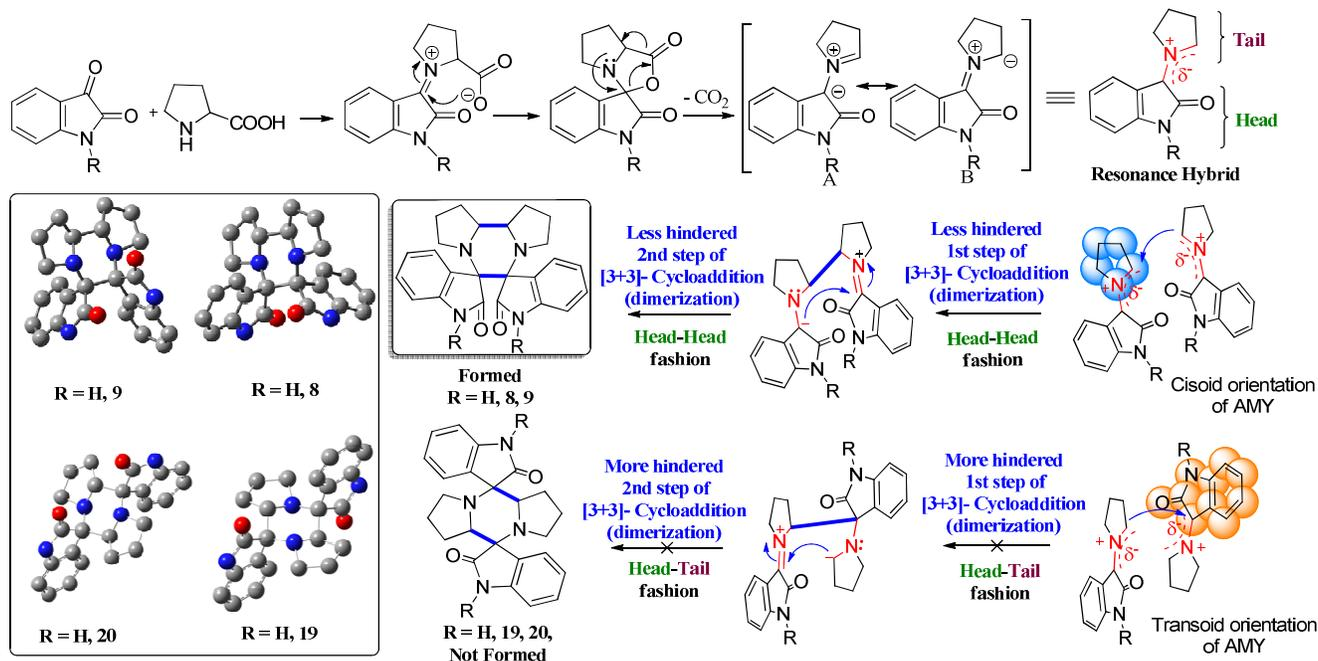
50 **Scheme 2.** Proposed mechanism of AMY generation and its dimerization.
