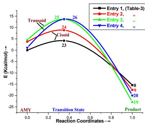
**Figure 3:** Energy profile diagram of [3 + 3] dimerization reaction of isatin – proline derived AMY.
