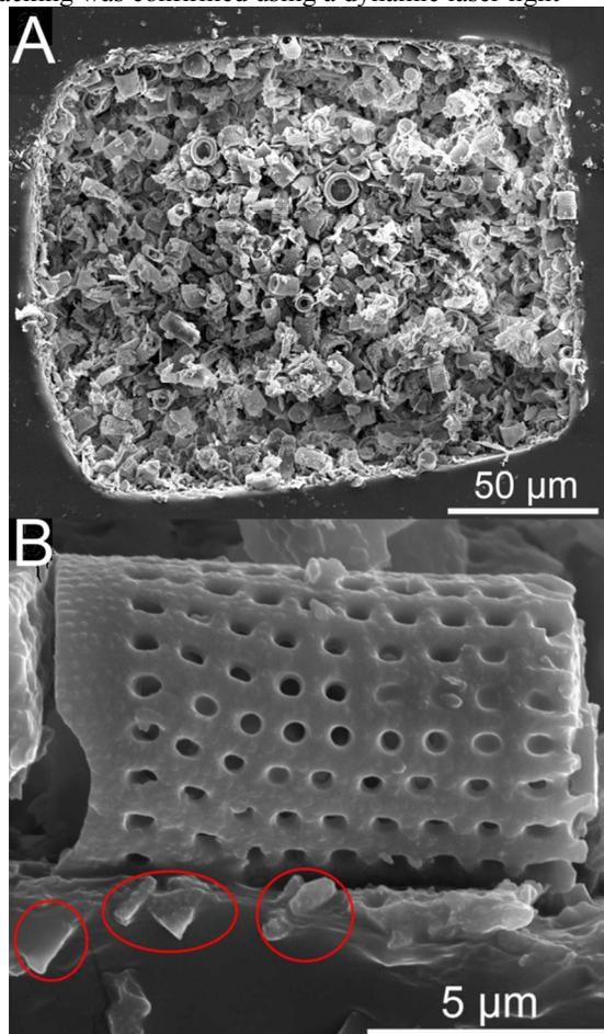
**Fig. 2** (A) SEM images of cross section of the packed channel and (B) SEM image of typical structure of a single DE particle (frustule) in contact with the PDMS wall showing intact packing of the particles.
