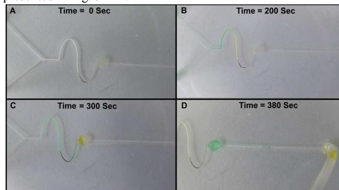
**Fig. 3** Time scan light microscopic images taken during separation process: (A) 0 sec of dye injection, (B) at 200 sec the dyes have been separated in DE packed channel, (C) at 300 sec the first separated yellow dye has occupied the detection area and (D) both the dyes have separated from each other.
