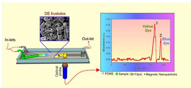
A simple frit-free PDMS (polydimethylsiloxane) microfluidic chromatographic separation and detection device, packed with diatomaceous earth (DE) microparticles as a normal phase stationary material using iron oxide magnetic nanoparticles is described.
