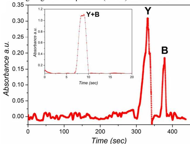
**Fig. 4** Functional characterization of fabricated microchip separation device showing typical chromatogram of two separated model molecules (blue and yellow dyes) using on-chip detection by UV/Vis microfiber optical probe: Inset is the chromatogram of mixed dye when injected without the DE stationary phase in the microfluidic channel, showing no separation.
