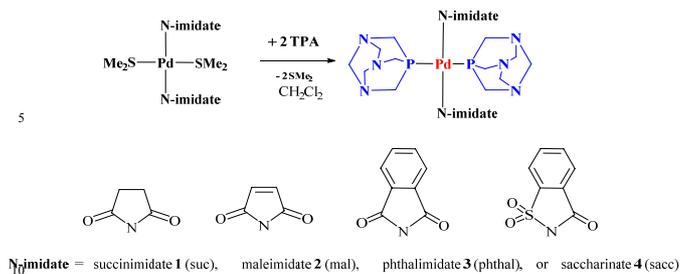
**Scheme 1:** Synthetic route for novel [Pd(Imidate)<sub>2</sub>(PTA)<sub>2</sub>] complexes.
