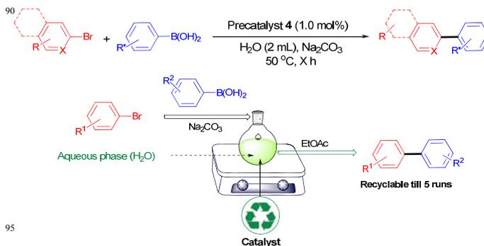
**Scheme 2:** Suzuki-Miyaura cross-coupling of aryl halides using [Pd(Imidate)<sub>2</sub>(PTA)<sub>2</sub>] complexes.
