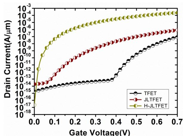
Fig. 4. Comparison of transfer characteristics of Si-TFET, Si-JLTFET and Si: Ge H-JLTFET with same dimensional parameters
