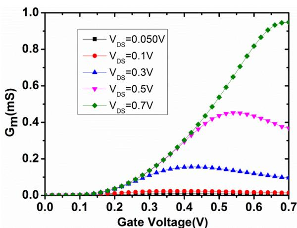
Fig. 7. Transconductance,  $G_m$  versus Gate voltage for H-JLTFET at  $V_{DS}$  from 0.05V to 0.7V
