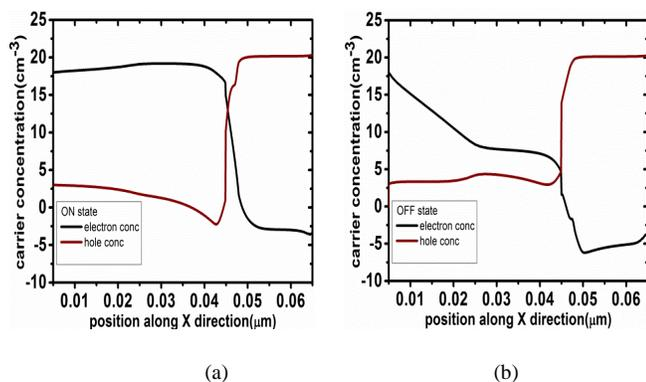
Fig. 3. Electron and Hole Concentration Profile of H-JLTFET as function of position along the x-direction in (a) ON state ( $V_{DS} = 0.7V$ ,  $V_{GS} = 0.7V$ ) (b) OFF state ( $V_{DS} = 0.7V$ ,  $V_{GS} = 0V$ ) at channel and  $HfO_2$  interface
