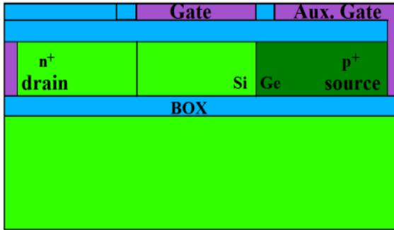
Fig. 1. Cross sectional view of device structure of Si: Ge Hetro-Junctionless Tunnel Field Effect transistor
