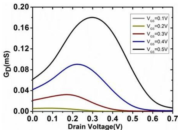
Fig.8. Drain conductance,  $G_D$  vs.  $V_{DS}$  at  $V_{GS}$  from 0.1 to 0.7V for H-JLTFET
