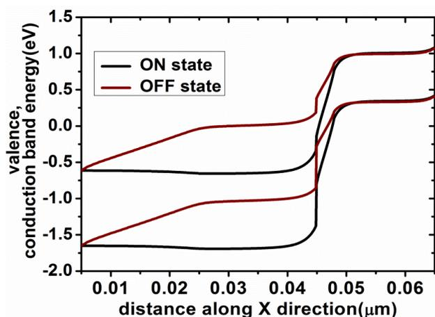
Fig. 2. Energy band diagrams taken horizontally across the channel of heterostructure bulk junction less tunnel FET, in ON state ( $V_{DS} = 0.7V$ ,  $V_{GS} = 0.7V$ ) and OFF state ( $V_{DS} = 0.7V$ ,  $V_{GS} = 0V$ ) along X direction at channel and  $HfO_2$  interface for H-JLTFET
