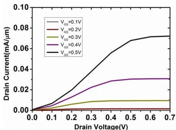
Fig. 6. Output characteristics at  $V_{GS}$  from 0.1 to 0.7V for H-JLTFET
