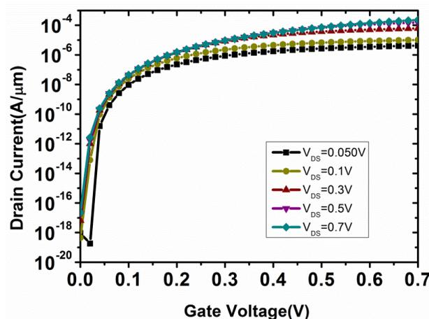
Fig. 5. Drain current versus Gate voltage for H-JLTFET at  $V_{DS}$  from 0.05V to 0.7V
