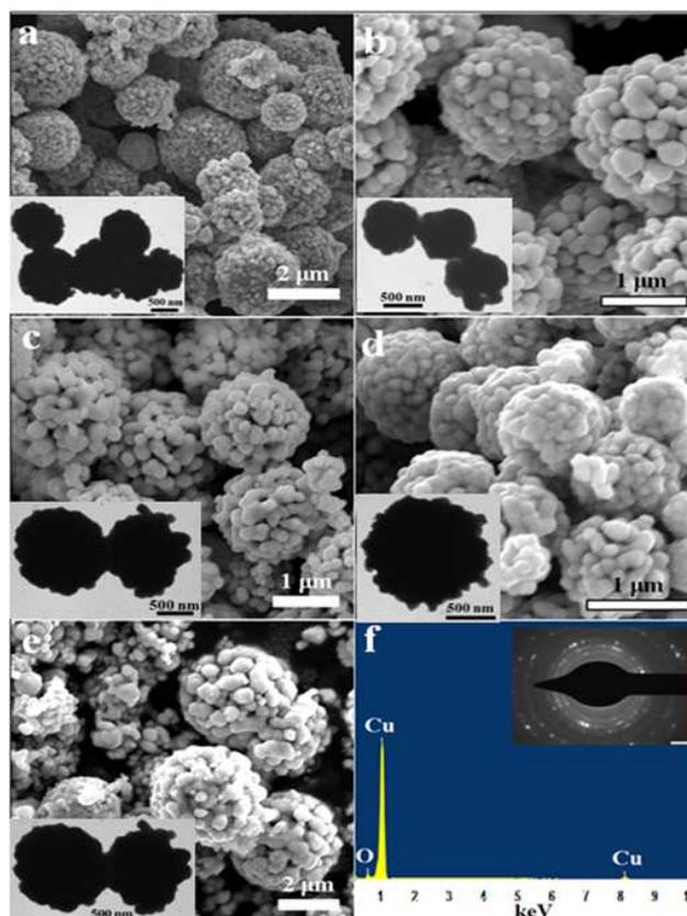
**Fig. 3** a-e) FEG-SEM images (insets are TEM images) f) EDS spectrum (inset SAED pattern) of Cu/Cu<sub>2</sub>O NMPs at 600 W for 2 min.
