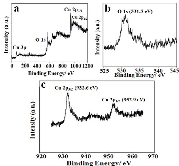
**Fig. 11** a) XPS survey spectrum b) O 1s region c) Cu 2p<sub>3/2</sub> region for Cu/Cu<sub>2</sub>O NMPs
