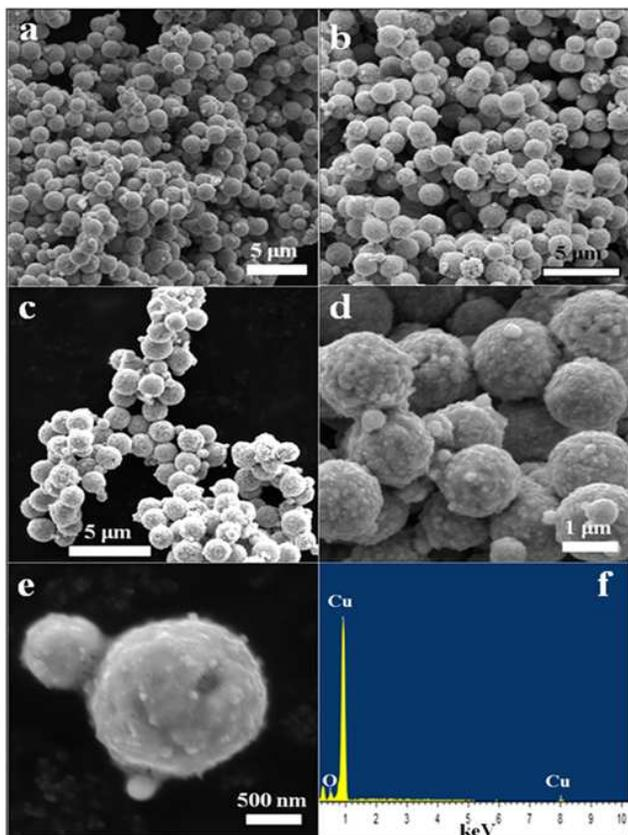
**Fig. 5** a-e) FEG-SEM images f) EDS spectrum of Cu/Cu<sub>2</sub>O NMPs at 600 W for 5 min.
