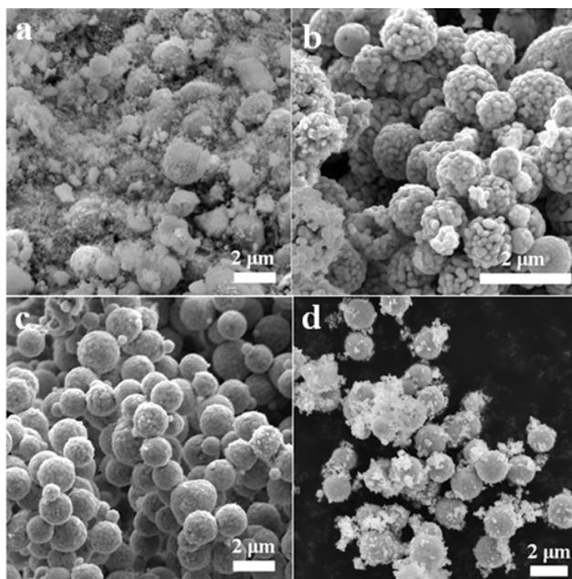
**Fig. 7** Growth of Cu/Cu<sub>2</sub>O NMPs a) at 360 W for 2 min b) 600 W for 2 min c) 600 W for 5 min d) 800 W for 2 min
