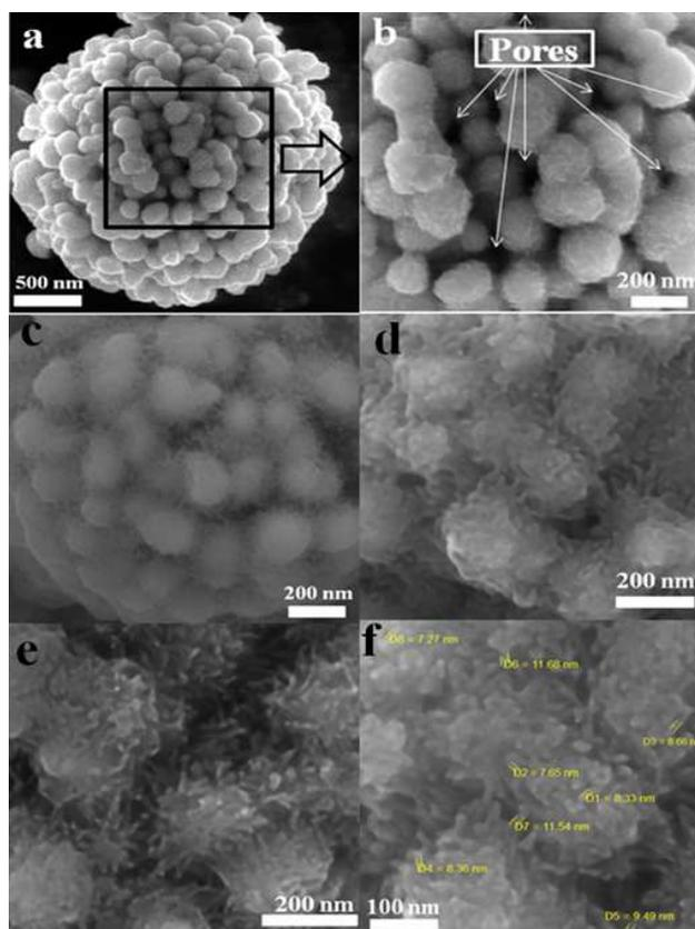
35 **Fig. 4** Magnified SEM images of Cu/Cu<sub>2</sub>O NMPs at 600 W for 2 min.
