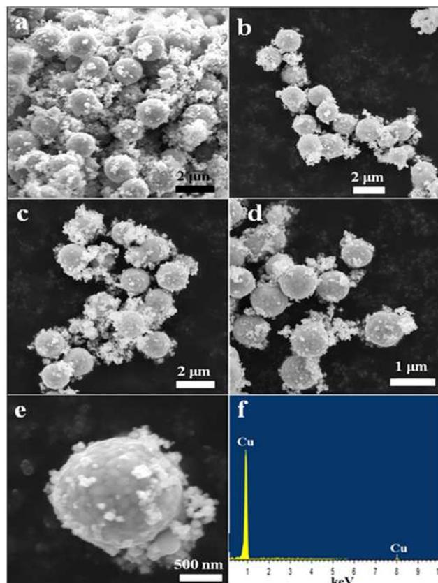
**Fig. 6** a-e) FEG-SEM images f) EDS spectrum of Cu/Cu<sub>2</sub>O NMPs at 800 W for 2 min.
