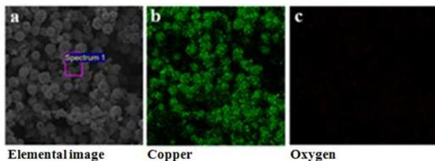
**Fig. 8** EDS composition mapping a) FEG-SEM image b) Copper (green) c) oxygen (red) for Cu/Cu<sub>2</sub>O NMPs at 600 W for 2 min.
