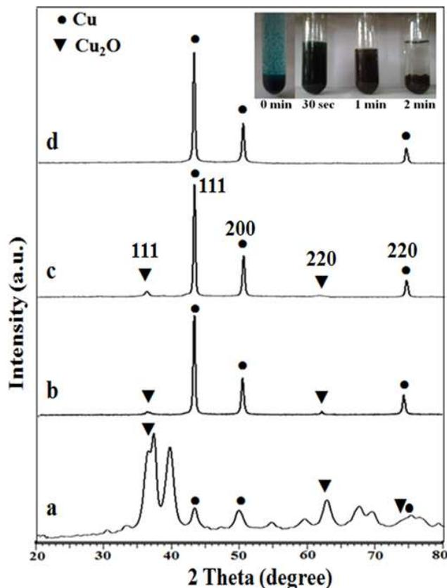
**Fig. 1** XRD pattern of Cu/Cu<sub>2</sub>O NMPs a) at 360 W for 2 min b) 600 W for 2 min c) 600 W for 5 min d) 800 W for 2 min with reaction progress observed by colour change (inset)
