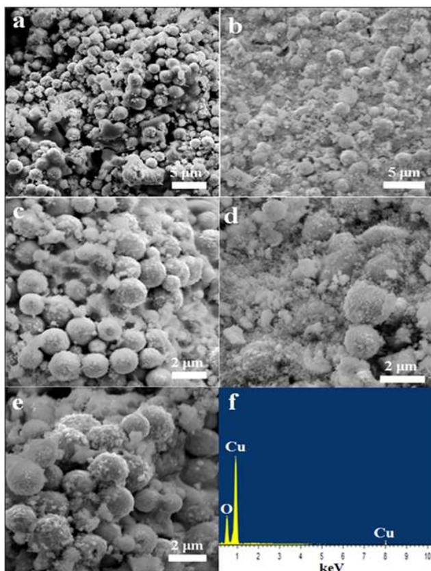
**Fig. 2** a-e) FEG-SEM images f) EDS spectrum of Cu/Cu<sub>2</sub>O NMPs at 360 W for 2 min.
