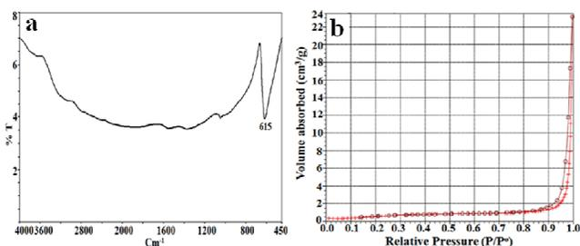
**Fig. 10** a) FT-IR spectra b) N<sub>2</sub> adsorption-desorption isotherm of Cu/Cu<sub>2</sub>O NMPs at 600 W for 2 min.
