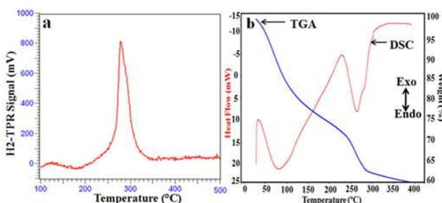
**Fig. 9** a) H<sub>2</sub>-TPR spectrum b) DSC/TGA graph of Cu/Cu<sub>2</sub>O NMPs at 600 W for 2 min.
