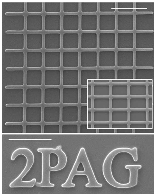
Fig. 6 SEM images of a \mu -grid and a Logo fabricated upon excitation at 800 nm ( P > 15 \text{ mW} , v = 5 \mu\text{m s}^{-1} ). Inset: Tilted view ( \theta = 45^\circ ). Formulation: SU-8 resin with Meta-Bz (0.4 wt %). Scale bars: 20 \mu\text{m} .
