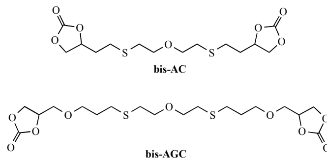
Figure 19 Chemical structures of the bicyclocarbonates 4,4'-(((oxybis(ethane-2,1-diyl))bis(sulfanediy))bis(ethane-2,1-diyl)bis(1,3-dioxolan-2-one) ( bis-AC ) and 4,4'-(2,9,16-trioxo-6,12-dithiaheptadecane-1,17-diyl)bis(1,3-dioxolan-2-one) ( bis-AGC ).
