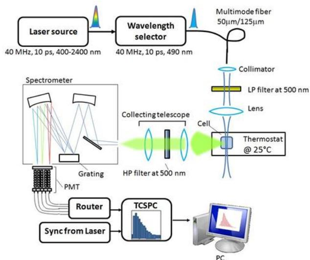
**Fig.8** Experimental set-up of fluorescence lifetime measurements. HP: High-pass; LP: Low-pass; PMT: Photomultiplier tube; TCSPC: Time-Correlated Single Photon Counting.
