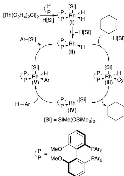
**Scheme 16. A proposed mechanism for Rh-catalyzed C–H silylation of arenes**
