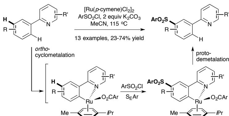
**Scheme 10. Ru-catalyzed *meta*-sulfonylation of 2-phenylpyridines**
