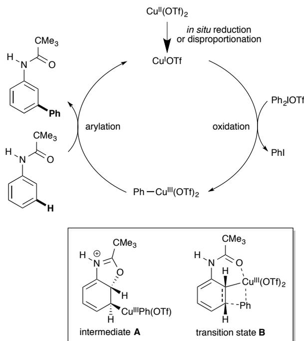
**Scheme 9. Proposed Cu(I)/Cu(III)-catalytic cycles for *meta*-C–H arylation**
