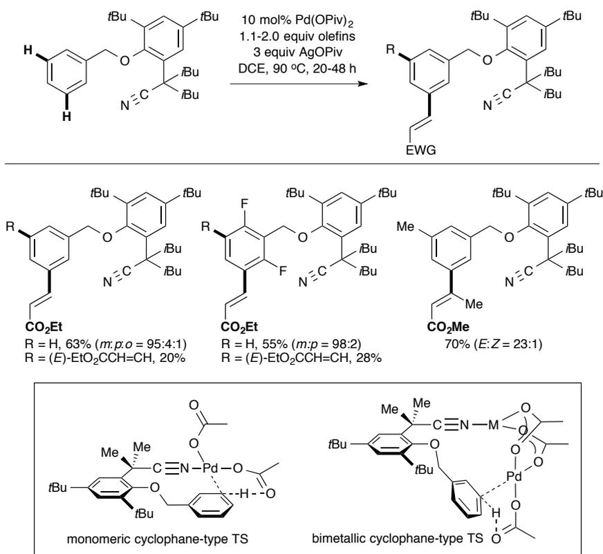
**Scheme 1.** Pd-catalyzed *meta*-C–H olefination using a nitrile end-on template
