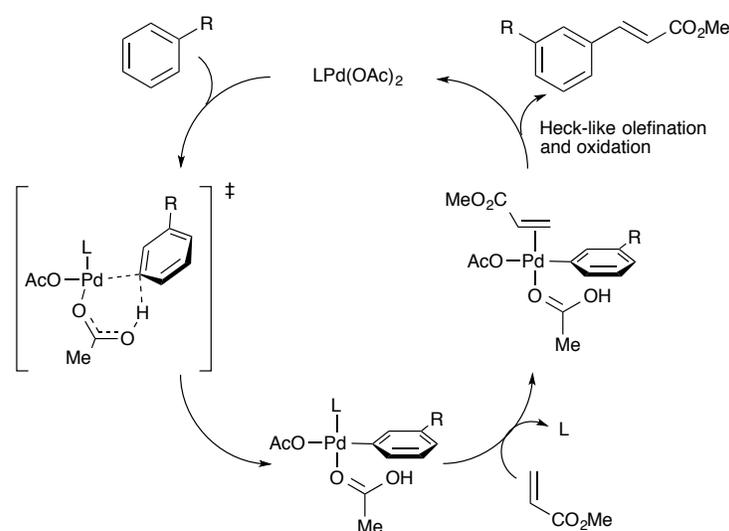
**Scheme 19. A proposed mechanism for Pd(II)-catalyzed C–H olefination**
