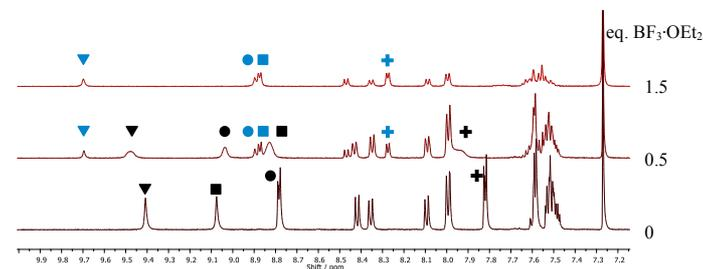
**Figure 2.** <sup>1</sup>H NMR spectral comparison of **1** (bottom) and **1**·BF<sub>3</sub> (top) in CDCl<sub>3</sub>. H<sup>a</sup> (▼), H<sup>b</sup> (■), H<sup>c</sup> (+) and H<sup>d</sup> (●) are indicated. Black markers indicate unmodified **1**, blue corresponds to **1**·BF<sub>3</sub>.
