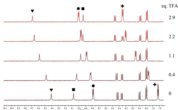
**Figure 4.** <sup>1</sup>H NMR spectral conformational analysis of switch **1** by chemical shifts of H<sup>a</sup> (▼), H<sup>b</sup> (■), H<sup>c</sup> (+) and H<sup>d</sup> (●) on the addition of TFA in CDCl<sub>3</sub>. The stoichiometry of TFA is calculated precisely by integration relative to an internal <sup>1</sup>H NMR standard.<sup>58</sup>
