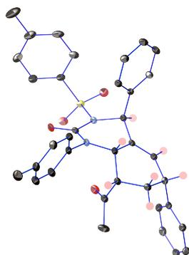
**Fig. 3**<sup>14</sup> Molecular structure of compound **6b** as an ORTEP plot. Thermal ellipsoids are shown at 30% probability level. Hydrogen atoms on the *p*-tolyl, phenyl, and methyl groups have been omitted for clarity.
