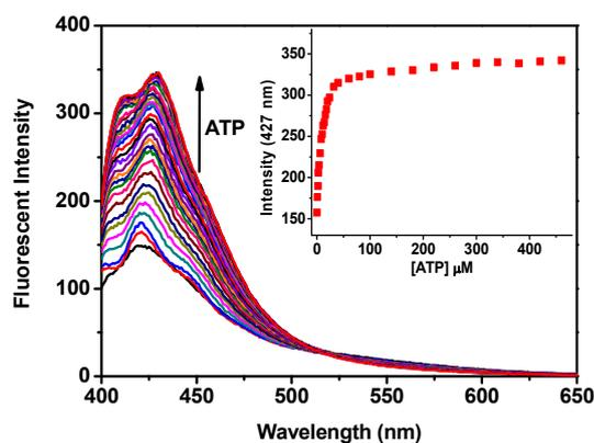
**Fig. 4** Fluorescent spectra changes of **1-2Zn** (10  $\mu\text{M}$ ) upon addition of ATP (0–450  $\mu\text{M}$ ) in the presence of  $\text{Na}_3\text{PO}_4$  (1000  $\mu\text{M}$ ) in aqueous solution of 10 mM HEPES buffer (pH 7.2) at 25  $^\circ\text{C}$  ( $\lambda_{\text{ex}} = 380 \text{ nm}$ ). Pot of fluorescent intensity changes at 427 nm against ATP concentrations is inserted.
