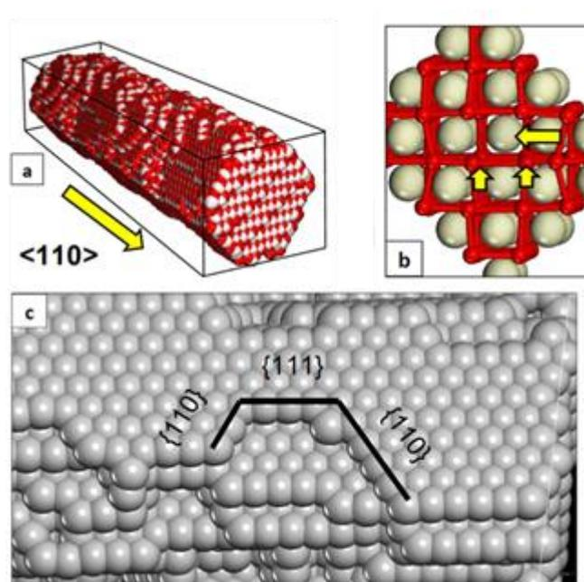
**Figure 8:** Atomistic structure of model ceria nanorods (a) perspective view of the nanorod showing the [110] growth direction and hexagonal nanorod cross-section (b) segment of (a) showing a defect cluster comprising one Ce vacancy and two oxygen vacancies as indicated by the yellow arrows. (c) Enlarged section of the surface of the nanorod (a) showing the steps, edges and corners and close packing of the cerium ions (oxygen ions are not shown).
