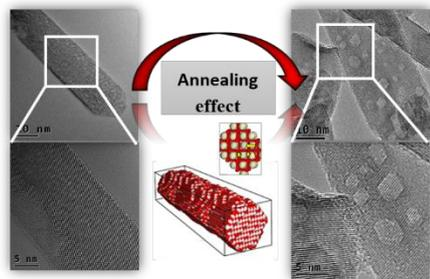
Annealing of cerium oxide nanorods results in the evolution of distinct cavities with polyhedral morphologies due to the high temperature activated rearrangement of cerium and oxygen atoms and vacancies on the as-synthesized nanorods.
