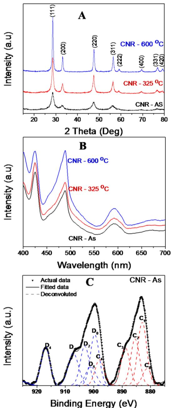
**Figure 1:** (A) Comparative XRD patterns of CeO<sub>2</sub> nanorods (CNRs) without annealing ("AS") and annealed at different temperature (325, and 800 °C) in air. (B) PL spectra of CeO<sub>2</sub> nanorods via excitation at 370 nm. (C) XPS Ce 3d spectra of as-synthesized CeO<sub>2</sub> nanorods.
