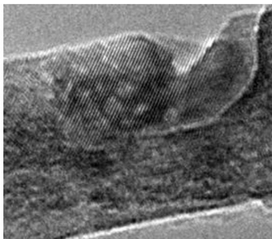
**Figure 5:** Formation of octahedral-projected patches in area of high-intensity electron beam irradiation (FEGTEM JEOL 2010F @ 200kV), along with general thinning and ablation, without any heating applied.
