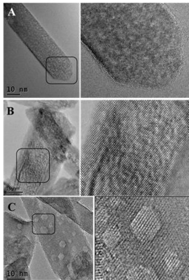
**Figure 2:** Ex-Situ annealing: HRTEM images, showing various amounts of imperfect crystallinity (image pairs with zoom-in of black rectangles): (A) as-synthesized CeO<sub>2</sub> nanorod. Rod-direction <110>. (B) Sample annealed at 325 °C in air. (C) Annealed at 800 °C: The rod-direction for (B,C) is <211>. The viewing directions for (A-C) are of <110> type. (JEOLJEM 3100-R005 @300kV)
