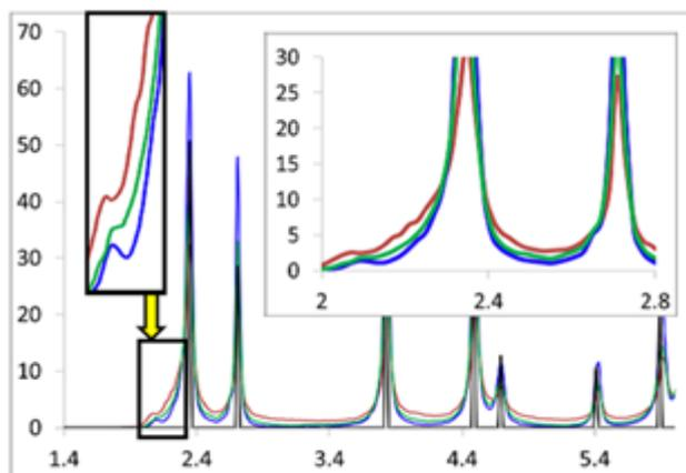
**Figure 9:** Radial distribution function (RDF) calculated for the three nanorods showing the considerable deviation of the Ce-O bond distances from those found in the bulk parent material; the RDF of bulk ceria is shown to compare. Abscissa: Ce-O interatomic separation (Å); ordinate:  $g(r)$ . Red trace: nanorod with grain-boundary; green trace: nanorod with growth direction along [110]; blue trace: nanorod with growth direction along [211]; black trace: parent bulk material.
