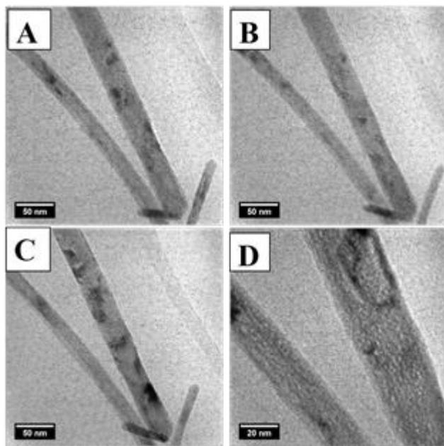
**Figure 3:** In-situ annealing: TEM images of CeO<sub>2</sub> nanorods mounted in heating holder. (A) at room temperature, (B) 80 minutes in-situ heated at 325 °C, (C+D) 80 min annealed at 600 °C, and cooled down to RT, and then again 180 min annealed at 600 °C (totally 80 + 180 minutes, the experiment was done over two days) (JEOL JEM 3010 @300kV).
