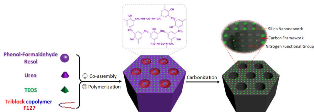
**Fig. 1** Schematic diagram of the procedure for preparation of nitrogen-doped ordered mesoporous carbon/SiO<sub>2</sub> nanocomposite.
