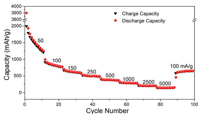
**Fig. 5** Capacity over cycling of the N-OMC/SiO<sub>2</sub> nanocomposite electrode at various current densities.
