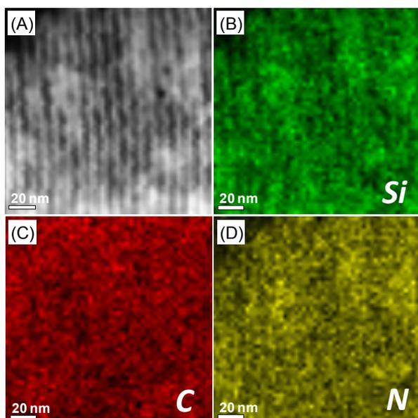
**Fig. 3** (A) HAADF-STEM image of N-OMC/SiO<sub>2</sub> nanocomposite, and (B~D) its corresponding EDX elemental mapping: (B) silica, (C) carbon, (D) nitrogen.
