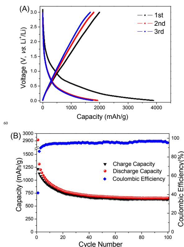
**Fig. 4** Electrochemical performance of the N-OMC/SiO<sub>2</sub> nanocomposite electrode: (A) charge/discharge profiles in the first three cycle measured at 100 mA/g, and (B) cyclability and Coulombic efficiency at 200 mA/g.
