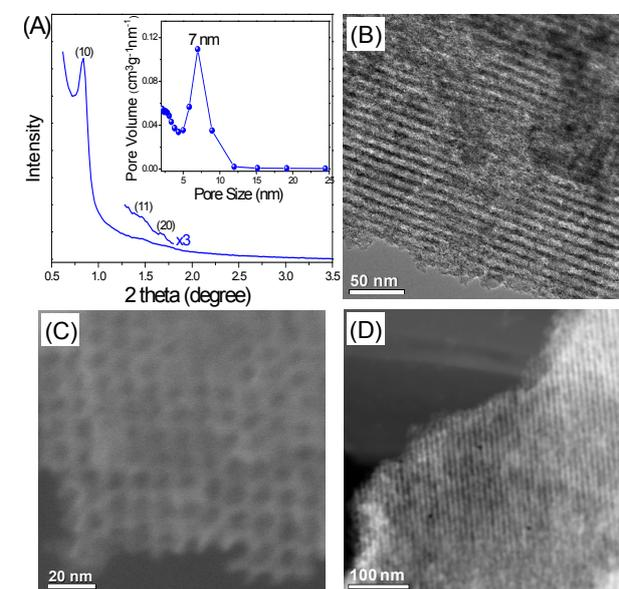
**Fig. 2** (A) Low-angle XRD pattern and BJH pore size distribution (inset), (B) TEM image, (C) SEM image and (D) HAADF-STEM image of N-OMC/SiO<sub>2</sub> nanocomposite.
