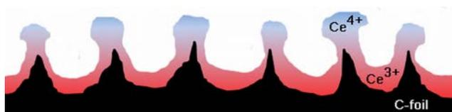
**Fig. 7.** Schematic layout of cerium ions in thicker layers of cerium oxide deposited by magnetron sputtering on the C-foil.
