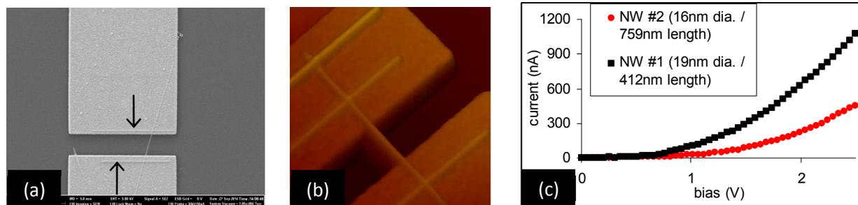
Figure 2. (a) SEM image of an assembled nanowire with arrows pointing to top-side EBID Pt contacts. (b) AFM image of a representative NW. (c) I-V plots from 2 nanowire samples. These are used to extract the contact resistance and NW conductivity to be 182.2 S/m and 145.7k $\Omega$ , respectively.
