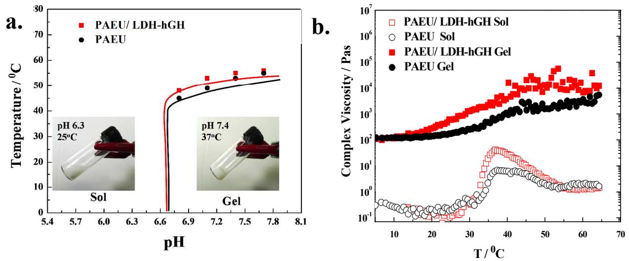
**Figure 5:** (a) Sol–gel phase transition diagram (b) Viscosity of 15 wt% pristine PAEU copolymer and its indicated nanohybrids solutions as a function of temperature at different pH.
