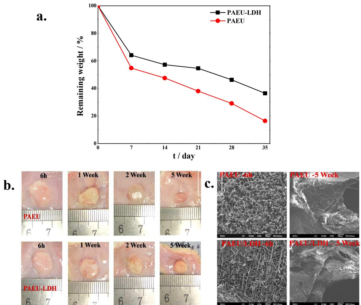
**Figure 7:** (a) *In vivo* degradation of PAEU and PAEU/LDH hydrogel (15 wt%, pH 6.3) determined by the mass loss method, (b) optical micrograph, and (c) SEM morphology of PAEU and PAEU/LDH hydrogels before and after degradation.
