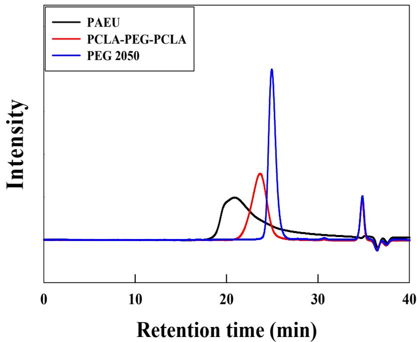
**Figure 2:** Gel permeation chromatography (GPC) of the synthesized PCLA-PEG-PCLA, PEG-2050, and multiblock copolymer PAEU.
