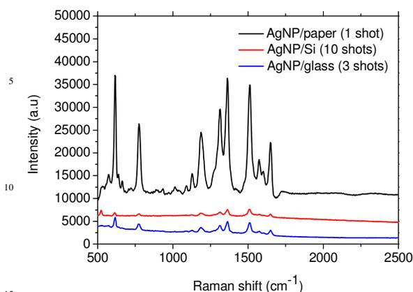
**Fig. 4** SERS spectra of 20- $\mu$ L R6G ( $10^{-6}$  M) droplets that had been dried on various hydrophobic SERS substrates.
