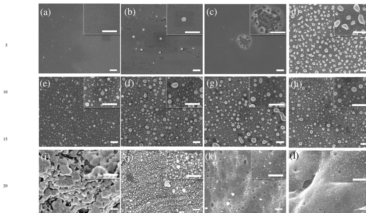
**Fig. 2** SEM images of the distributions of Ag NPs formed on (a–d) Si, (e–h) glass, and (i–l) filter paper after different numbers of shots of KrF laser illumination. For Si and glass, the numbers of shots were (from left to right) 1, 3, 5, and 10; for filter paper, the numbers of shots were (from left to right) 0, 1, 3, and 5. Inset: Enlarged images of the NPs. Scale bars: (a–h) 1  $\mu\text{m}$ ; (i–l) 200 nm.
