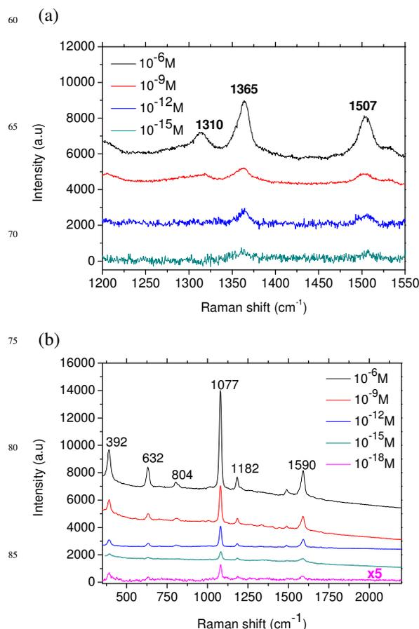
**Fig. 7** SERS spectra of various concentrations of (a) R6G and (b) 4-ATP dried on Ag NP-containing SERS filter paper, demonstrating attomolar detection ability.
