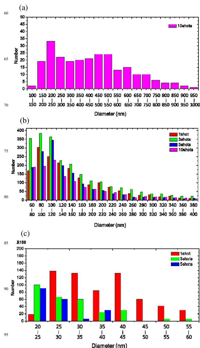
Fig. 3 Particle size distribution within a  $10 \times 10 \mu\text{m}^2$  area of Ag NPs formed on (a) Si, (b) glass, and (c) filter paper.
