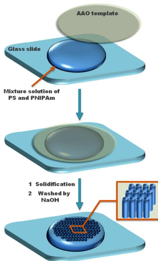
Figure 1 A typical process on preparing the bioinspired responsive nanocupule surface.
