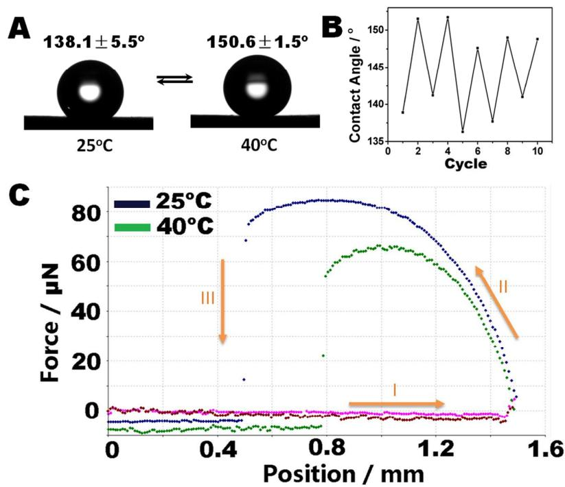
Figure 3 A) contact angle changes of the nanocupule surface at 25°C and 40°C; B) the repeatability of the fabricated film; C) the adhesion force of the prepared film at 25°C and 40°C, on which the maximum values were 85μN and 65μN, correspondingly.
