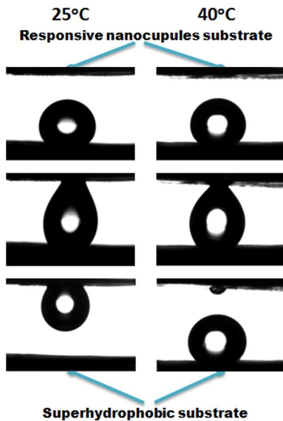
Figure 4 A application of the responsive nanocupule surface on the water selection. 8mg water droplet was placed on a superhydrophobic substrate, the droplet could be caught up at 25 °C; when the temperature was increased to 40 °C, it could not be caught up.
