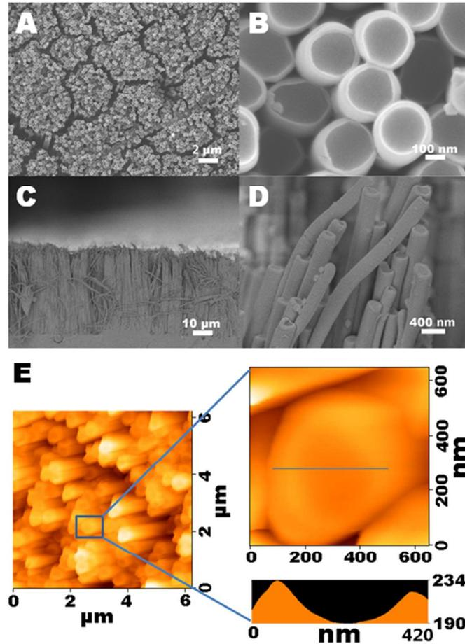
Figure 2 A) and C) the SEM images of the prepared nanocupule surface in top and profile view, respectively; B) and D) the magnified ones correspondingly; E) the AFM image of the prepared surface, which showed the diameter and depth of each cupules were 284nm and 38nm individually.
