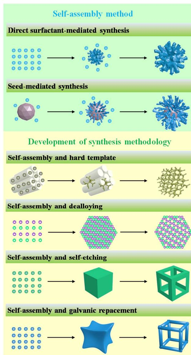
**Fig. 3** Various methods based on self-assembly for the synthesis of nanoporous metal nanocrystals.
