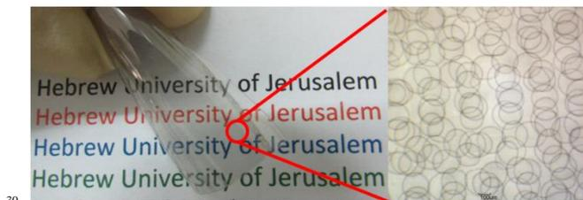
**Fig. 5** Flexible CNT TCF formed by inkjet-printed CNT rings.
