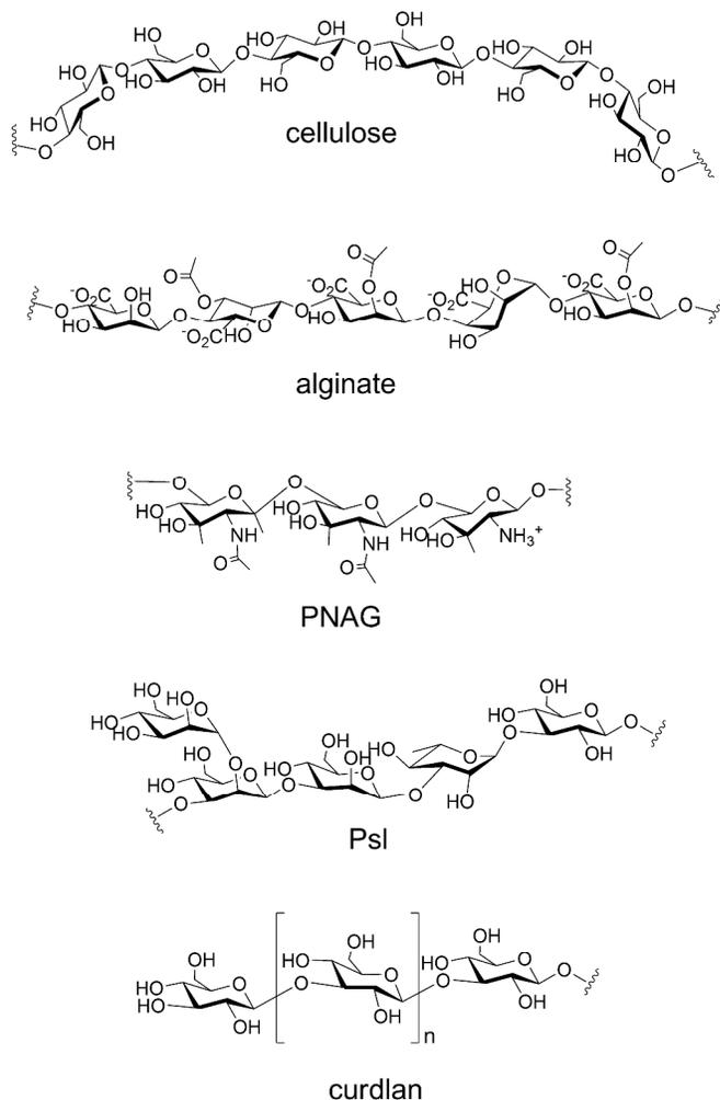
**Fig. 2.** Chemical structures of cellulose, alginate, Psl and 2,3 - poly- $\beta$ -1,6-N-acetylglucosamine (PNAG) and curdlan polysaccharides.
