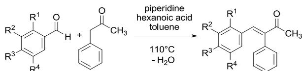
Scheme 1 The synthesis of 3,4-diphenylbut-3-en-2-one derivatives
