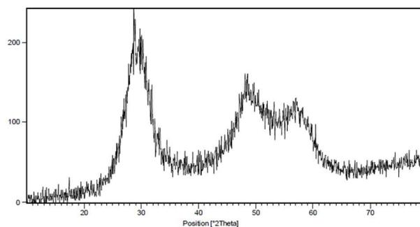
Fig. 3 XRD spectrum of ZnS nanoparticles
