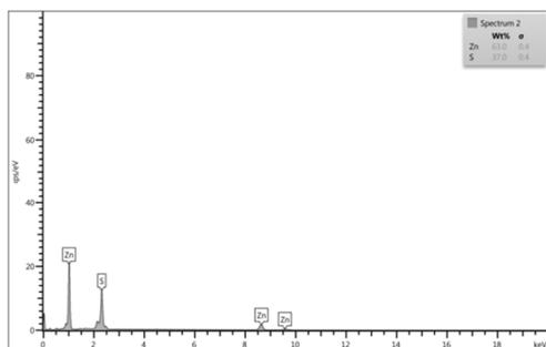
Fig. 5 The EDX spectrum of ZnS NPs catalyst
