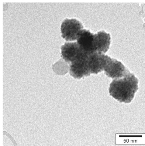
**Fig. 9** TEM image of ZnS nanoparticles after five subsequent runs
