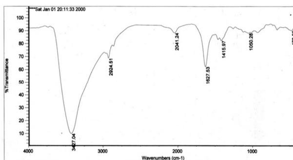
Fig. 2 The FT-IR Spectrum of ZnS NPs catalyst
