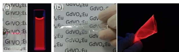
Fig. 3 Photographs of (a) aqueous colloidal suspension (The light beam was irradiated from the side to demonstrate the Tyndall effect.) and (b) PVA composite film containing GdVO 4 :Eu under day light and 254 nm UV irradiation.
