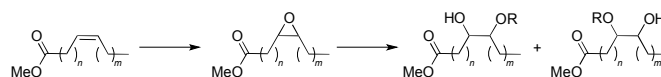
Scheme 1. General strategy for addition of functionality to a double bond in FAME, via ring opening of the epoxide with a carboxylic acid or alcohol nucleophile, leading to 2 regioisomers.
