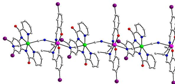
**Figure 3.** The asymmetry unit and one-dimensional chain structure of complex **3**. All the hydrogen atoms and solvent water molecules have been omitted for clarity.
