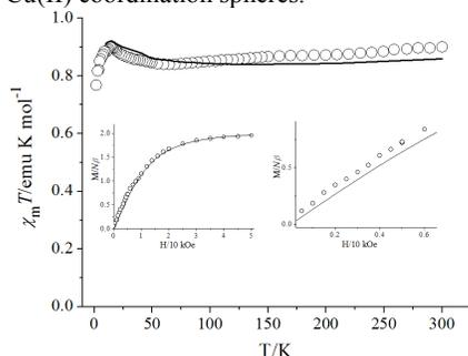
**Figure 8.** Temperature dependence of  $\chi_M T$  of complex **5**. The solid line represents the best fit based on the parameters discussed in the text. Inset: Field dependence of magnetization at 2 K (the dotted line is the Brillouin curve for uncoupled Fe(III) and Mn(II) ions with  $g = 2.0$ ).
