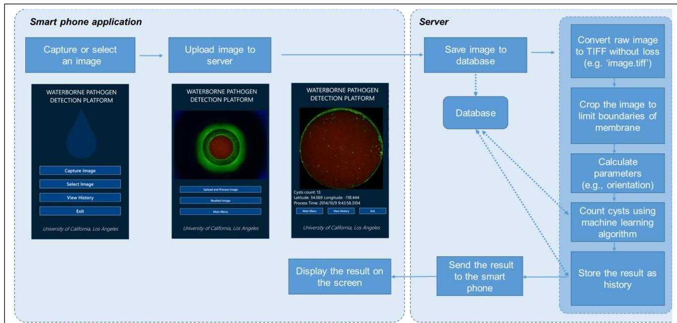
**Fig. 3** Process flow for automated detection and counting of *G. lamblia* cysts using our custom developed smart application running on a Windows-based mobile phone. The processed image and cyst counting results are sent back to the mobile phone within less than ~2 minutes.
