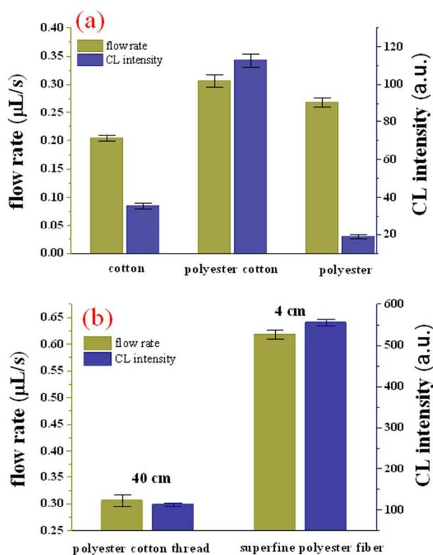
**Fig. 3** Effects of thread tail materials on siphonage flow rate and CL response. (a) Flow rate and CL response comparison among three thread tail materials of cotton, polyester cotton blend and polyester; All the tails
