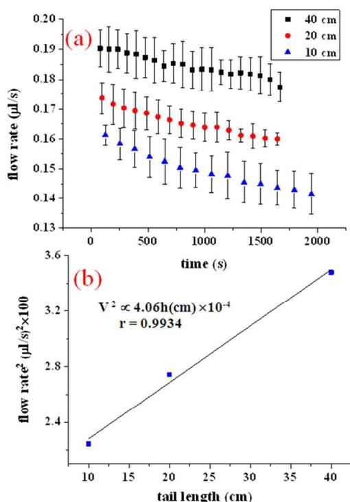
**Fig. 2** (a) Water flow rate as a function of time corresponding to the tail length of 10 cm, 20 cm and 40 cm polyester cotton blend tail; Error bars represent the  $\pm$  SD of triplicate measurements. (b) Depiction of the relationship between the square of flow rate and the length of tail.  $V$  is the average of flow rates with respect to each tail length;  $h$  is the thread tail length as well as the siphonage height difference;  $r$  is the linear correlation coefficient.
