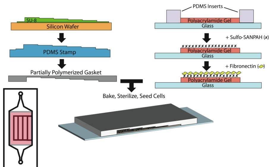
Figure 1. Device manufacture and preparation: the PDMS step gasket is constructed using traditional soft lithography techniques and then adhered to a coverslip containing a 100 nm height, rectangular-shaped polyacrylamide gel coated with fibronectin. Flow is applied through the device using a peristaltic pump connected to the inlet and outlet ports of the device.
