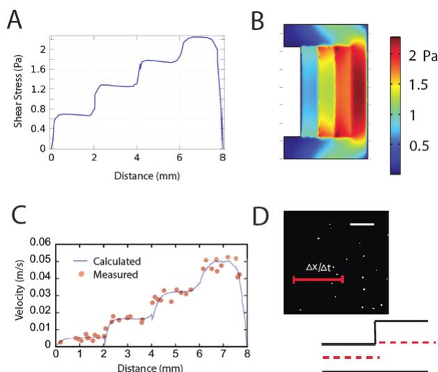
Figure 2. A) Estimated wall shear stress along the centerline of the step device using the finite element model. B) Accompanying wall shear stress contour C) Comparison of measured particle velocity and velocity magnitude predicted by the finite element model. D) Schematic of the validation approach: particles were measured at the half-height of each step (scale bar = 50  $\mu\text{m}$ ).
