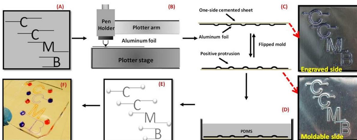
Fig. 1 Schematic illustration of the process for fabrication of microfluidic device (A) CAD design, (B) pattern/s transferred onto the aluminium foil using the X-Y pen plotter, (C) polyester film supported patterned foil as master, (D) molding of PDMS against patterned aluminium foil mold (E) molded PDMS after punching the access holes (F) Final PDMS devices sealed on glass surface.
