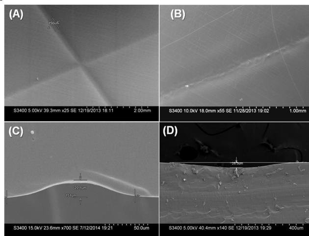
Fig. 2 SEM images of (A) PDMS replica of channel structure created by metal tip (B) PDMS replica of channel structure created by fibre tip and CS of shape of channel prepared using (C) metal tip and (D) fibre tip.
