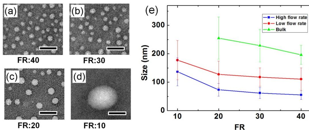
**Fig.3** TEM images of PLGA nanoparticles precipitated under different FRs. (a) middle channel: 10 mL/hr, each side channel: 200 mL/hr, and FR: 40, (b) middle channel: 13 mL/hr, each side channel: 198.5 mL/hr, and FR: 30, (c) middle channel: 20 mL/hr, each side channel: 195 mL/hr, and FR: 20, and (d) middle channel: 38 mL/hr, each side channel: 186 mL/hr, and FR: 10. The scale bar is 100 nm. (e) Size distribution of PLGA nanoparticles as a function of FR by different approaches.
